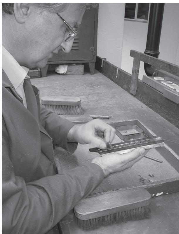
(Photo 5: After-treatment of the master). Scraping the cooled wax plate just leaving the conductive lines.
