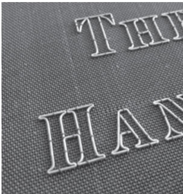
*(Photo 2 The handmade Note) This shows the traditional way of forming the copper wire, note how the mould maker has economized his work - if possible one letter is bent from one piece of wire.) Silkeborg Papirfabrik.*
