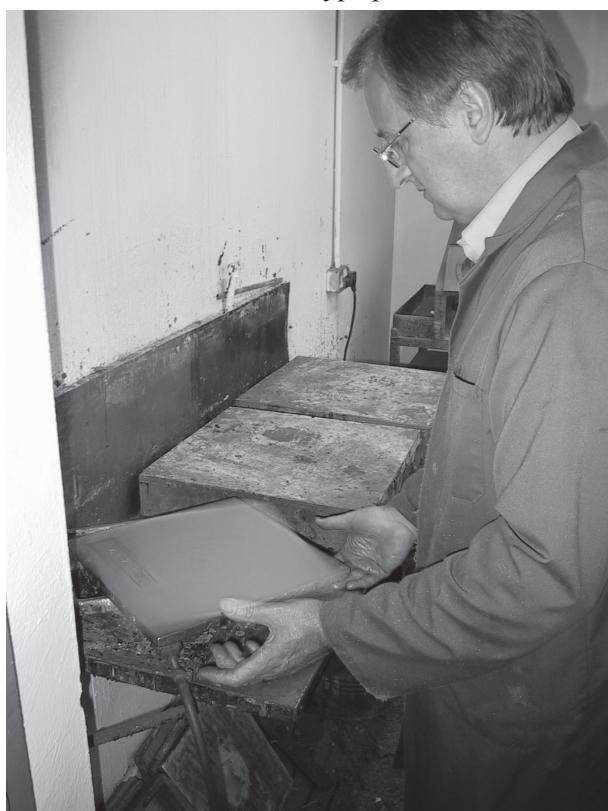
*(Photo3 Warming wax tablet) Rotating the wax tray over the flame. The impression seen already in the wax tablet is due to that Frank Jones first had demonstrated a 'light' version of the process, normally the tablet would be clean.*
