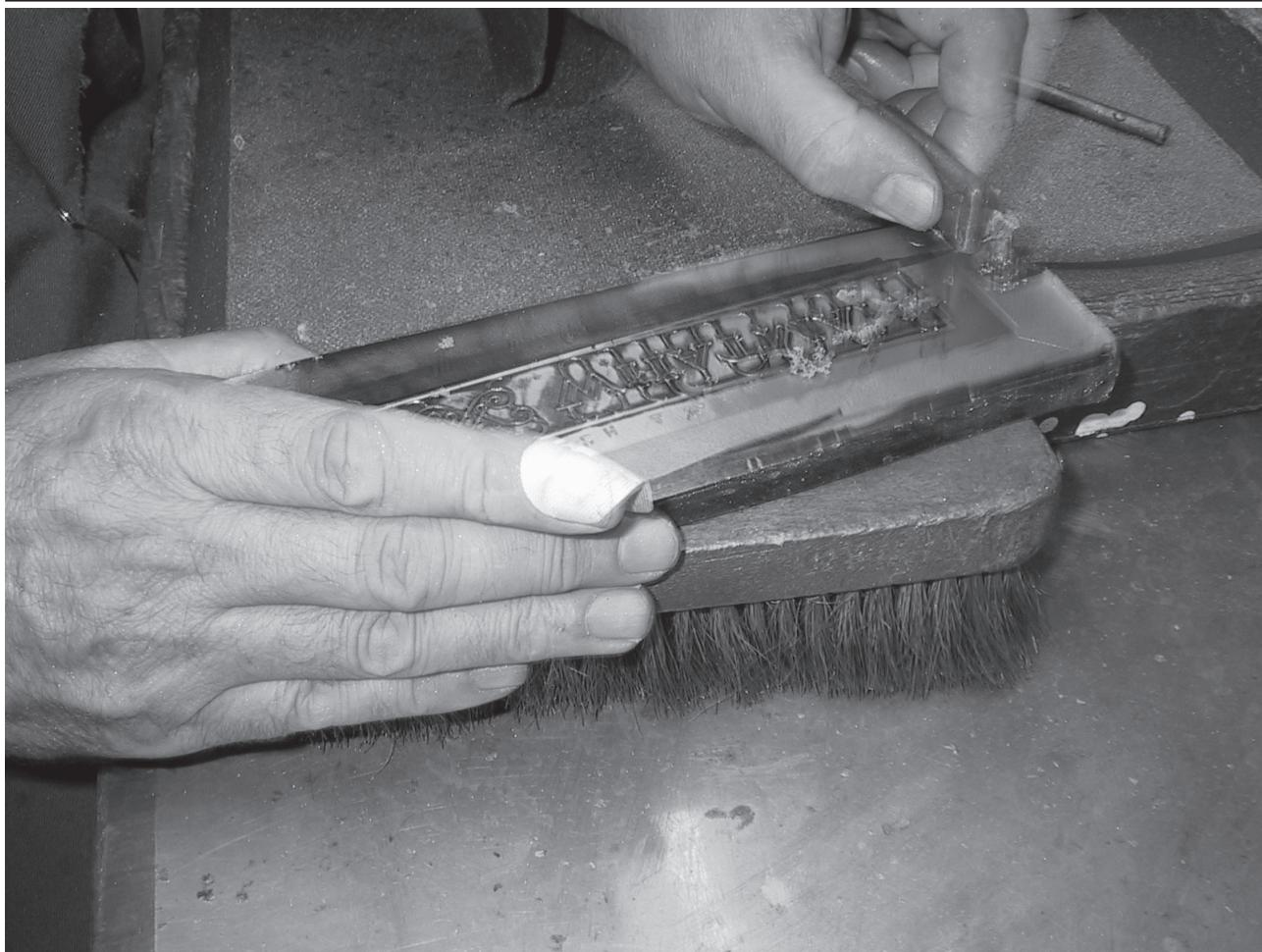
(Photo 6: After-treatment of the master). Close-up of the scraping and the scraping tool.
