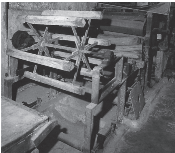
Fourdrinier machine from Amalfi with the system to roll the still wet paper before cutting.
