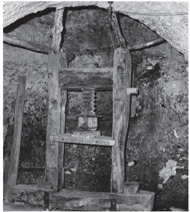
The 18 th century press of olive- and chestnut wood from Ferdinando Amatruda's paper mill
